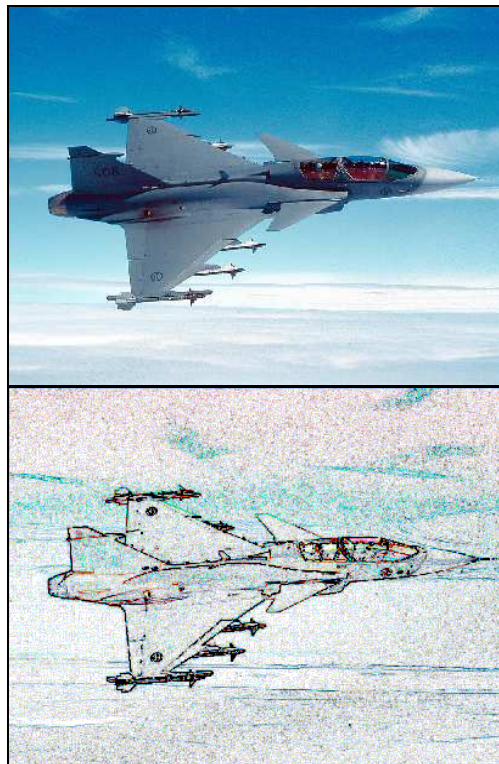
Fig. 11.2. An example of 2D image convolution – edge detection
